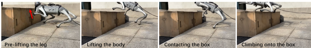
Figure 5: Climbing a wooden box with Lidar
